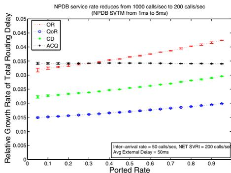
Fig. 2. Scenario I – Relative Growth Rate of Total Routing Delay
