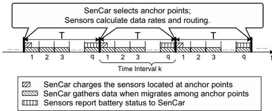
Fig. 1. Timing of joint mobile energy replenishment and data gathering (J-MERDG).
