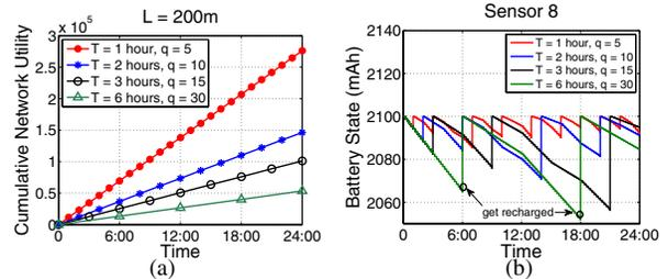
Fig. 5. Performance of J-MERDGD as the function of  $T$ . (a) Cumulative network utility. (b) Battery states of sensor 8.
