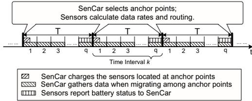
Fig. 2. Architecture of joint mobile energy replenishment and data gathering (J-MERDG).
