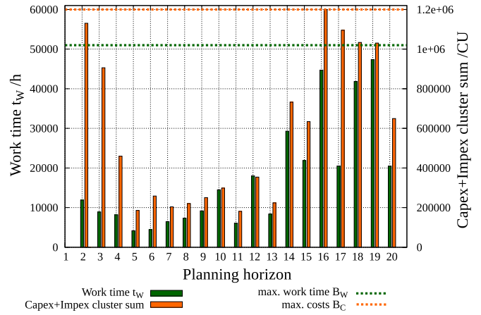
Fig. 9: Total cost and work time distribution limited by constraints (9-cluster Scenario, demand model A)
