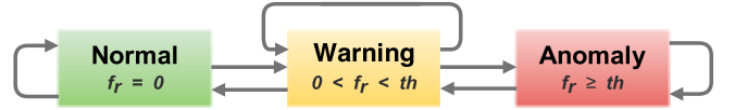
Figure 13. State machine of change detection output. f_r is the fraction of change notification in the shift register, th is the state transition threshold. Each symptomatic and diagnostic signal has its dedicated state machine.
