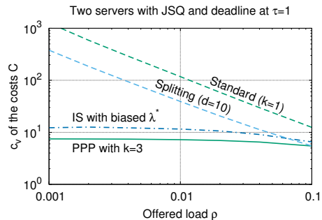
Fig. 6. Coefficient of variation of the random quantity C (the number of deadline violations in a busy period) with different simulation approaches.
